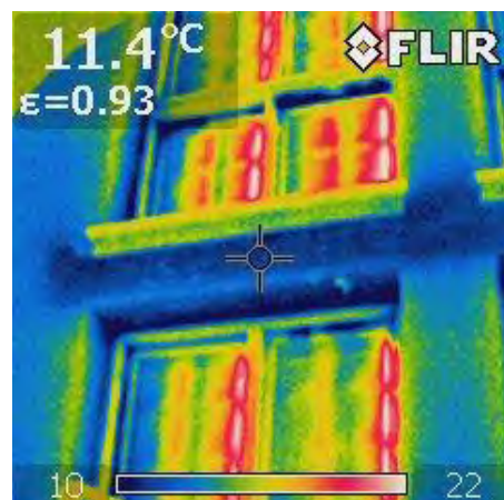
Photo 4 and IR photo 5. A severe damage at the first floor have appeared and the low surface temperatures is giving f = 0.71 just above the limit of risk for condensation and mould growth in the construction. Photo to the left by Maja Lindman and to the right by Heidi Norrström.
