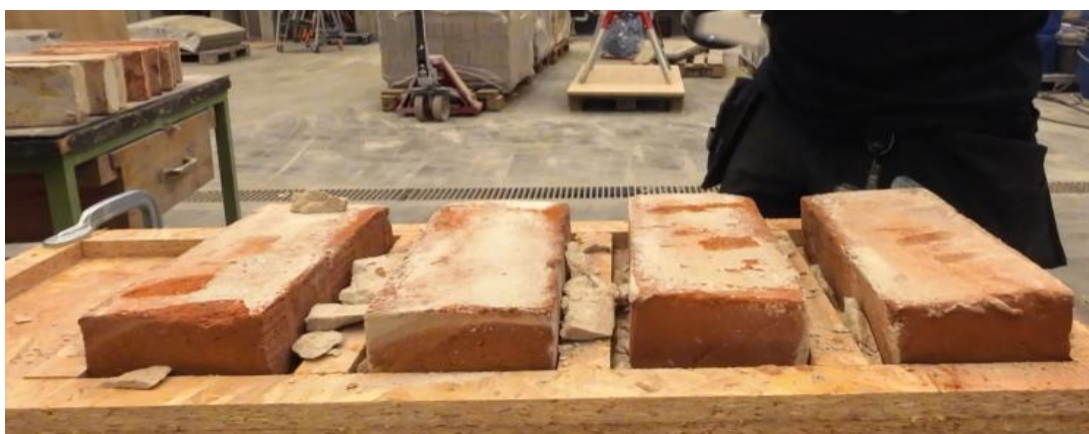
Figure 7: The bricks after cleaning with a chisel (taken by Rasmus Stenholt-Jacobsen)
