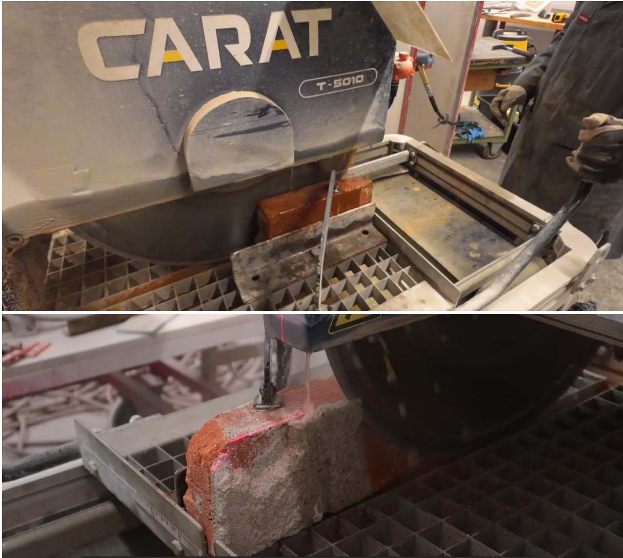
Figure 12: Cleaning of the brick by saw cutting with water (taken by Rasmus Stenholt-Jacobsen)
