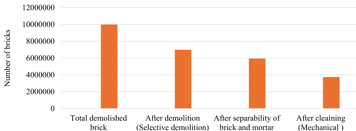
Figure 16: The diagram shows brick flow in the reuse process with selective demolition, separation, and mechanical cleaning
