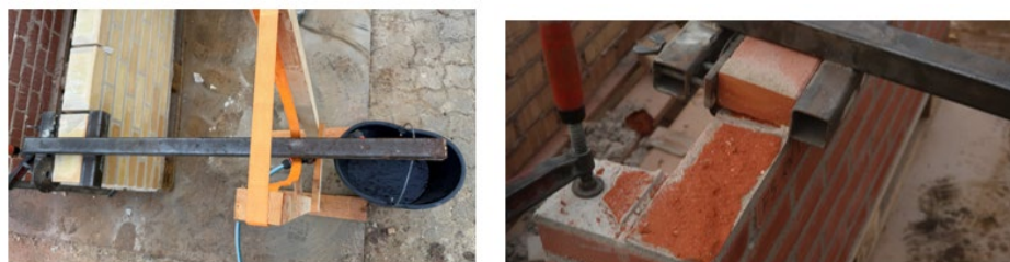
Figure 6. Test setup the so-called bond wrench to assess the bond strength between brick and mortar
