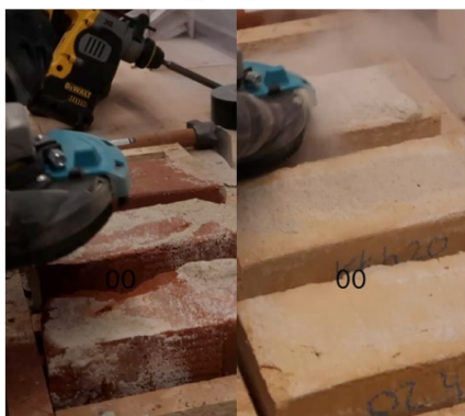
Figure 5. Examples of brick cleaning methods assessed within the project include power hammer, Paoloni oscillating chisel machine, angle grinding, and sawcutting
