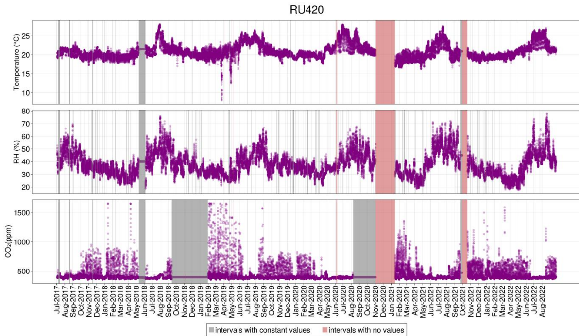
Figure 67 Temperature Relative humidity and CO 2 for the classroom 420. In the plot intervals with no values and intervals with constant values are highlighted. The minimum window size utilized for intervals with constant value was 12 hours.
